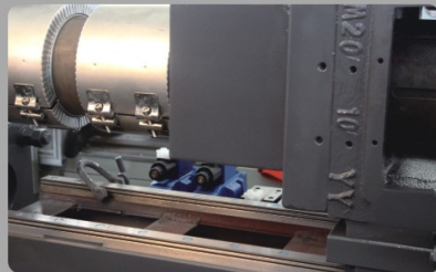
The linear guide rail supports the injection stand and guides its motion
